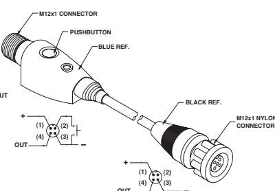
**AC132** Right-angle, M12 micro, 4-conductor, connector/cable assembly, 5 m (16') (for flat-profile connector-style sensors)
