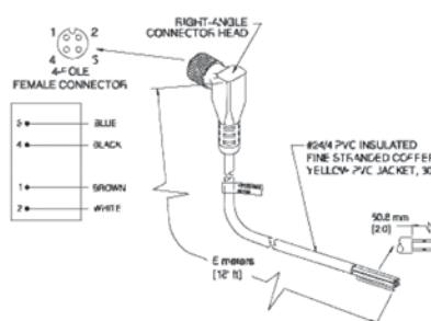
**PB100** In-line accessory push-button for teaching window limits (for Virtu series sensors).
